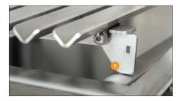
6 Place the V-channel surface onto the lift frame so that it sits securely on the lift frame. The open V-channel ends should be facing you as you stand in front of the grill, with a gentle slant toward you. Crank the surface to the top. Underneath the front of each surface are leveling 'feet' that can be flipped outward to eliminate the slant when required (such as for pot placement).
