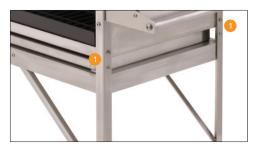
Gently set the grill body on its back onto a smooth surface. Using the hex key and bolts included affix each leg—two wheeled legs go on the back corners for our residential models while the Asadors have four with crossbraces. Lift each end of the grill as you attach the legs, then stand the grill upright.
