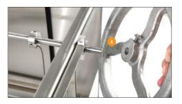
4 Slide the cast crankwheel onto the end of the crank axle that runs across the grill. Tighten the bolt at the neck of the wheel so that it meets the notch in the axle.
