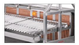
Asador models use floating fire brick heat shields which ship assembled. If you need to disassemble—remove the top bolts at the back and lift off the retaining cap. The bricks are stacked in columns, held in place with vertical t-shaped retainers. Once the cap is off the retainers and bricks can be removed. Keep careful track of the retainers for re-assembly.
